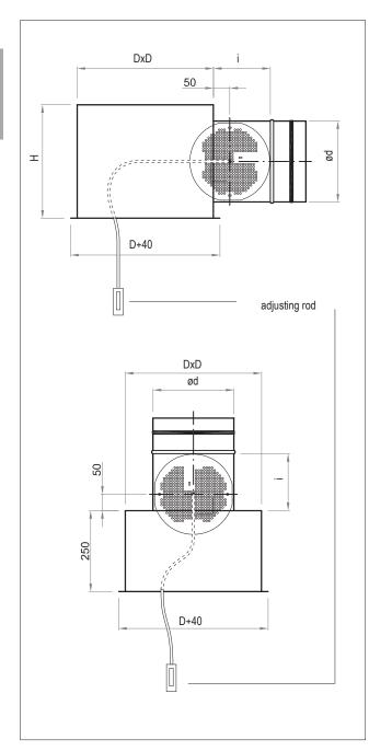
Expansion boxes can be connected to the ventilation installation through the side or top.
